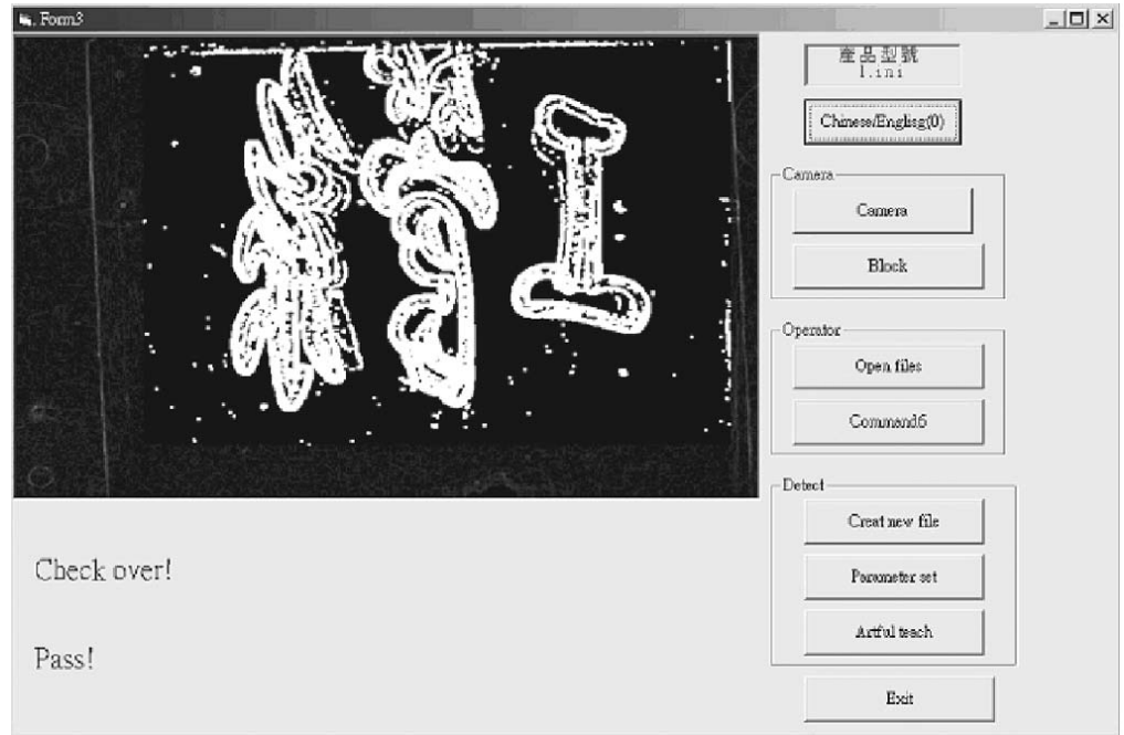
Fig. 14. HMI screen for color-grade inspecting cell
